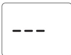
From the Frost Protection mode, press the **⊕/⊖** button twice. The unit shows 3 dashes. To return to Automatic mode or to Simple thermostat mode, press the **⊕/⊖** button again.
